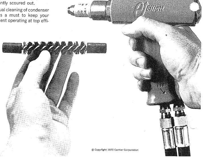
Connect the Jiffy Gun's two light flexible hoses to your air compressor (or a nitrogen bottle, over 1,000 tubes can be cleaned from just one commercial-sized bottle) and to your water supply. You're ready to clean tubes faster than you ever thought possible (about 20-25 tubes per minute). Load all the brushes in the tubes. (Time is money: brushes are reusable!) Fire!
